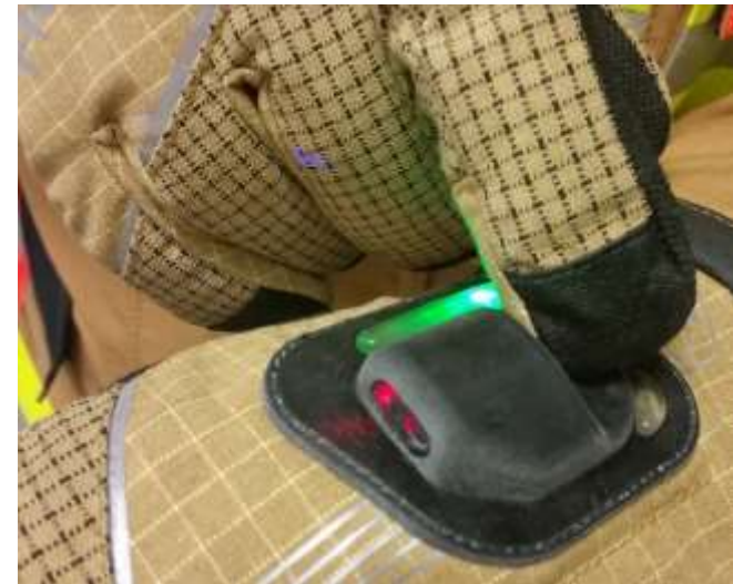
The 2 nd generation of the smart glove with integrated LED bar graph.
